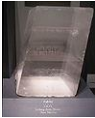
Calcite rhomb from Iceberg claim, Dixon, New Mexico showing double refraction .
